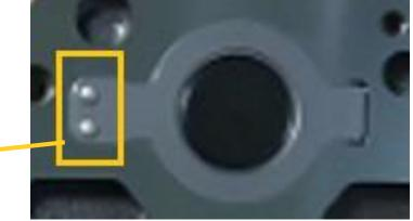
Suction reed riveted on valve plate
