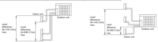
If the outdoor unit is positioned higher than the indoor units.
