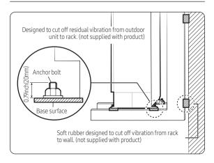
Install a proper grommet in order to reduce noise and residual vibration transferred by the outdoor unit towards the wall.
