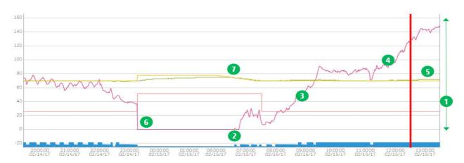
This logic works in reverse for heating. Heating Zone Demand analytic ranges from 0% to -163%.
