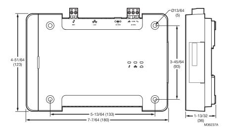
Fig. 1. Dimensions in in. (mm).
