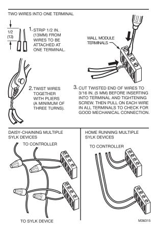
Fig. 6. Options for wiring multiple Sylk devices.
