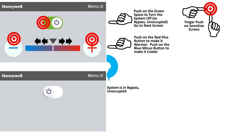
Using the new wall module. Going from Bypass (Unoccupied) to Occupied
