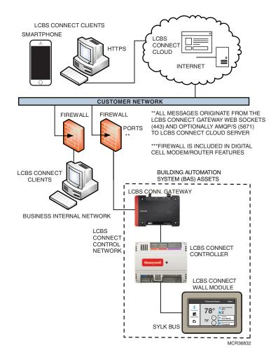
Fig. 1. Example: LCBS Connect system installed in a corporate network.
