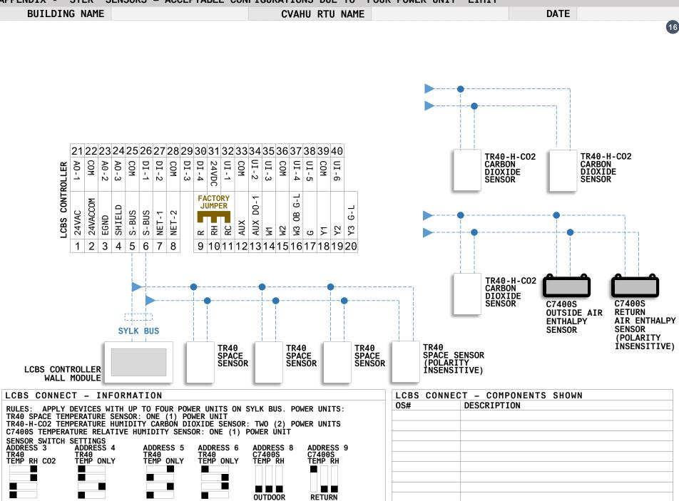
APPENDIX - "SYLK" SENSORS - ACCEPTABLE CONFIGURATIONS DUE TO "FOUR POWER UNIT" LIMIT
