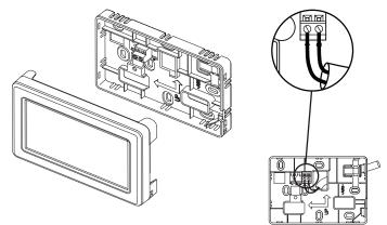
WARNING! Directly applying 24Vac to the wall module may cause damage to the device.
