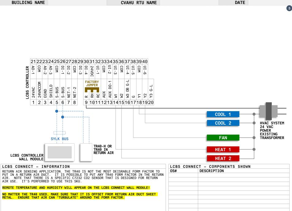
APPLICATION EXAMPLE 1 - RETURN AIR SENSING WITH STANDARD TWO HEAT TWO COOL CONTROL
