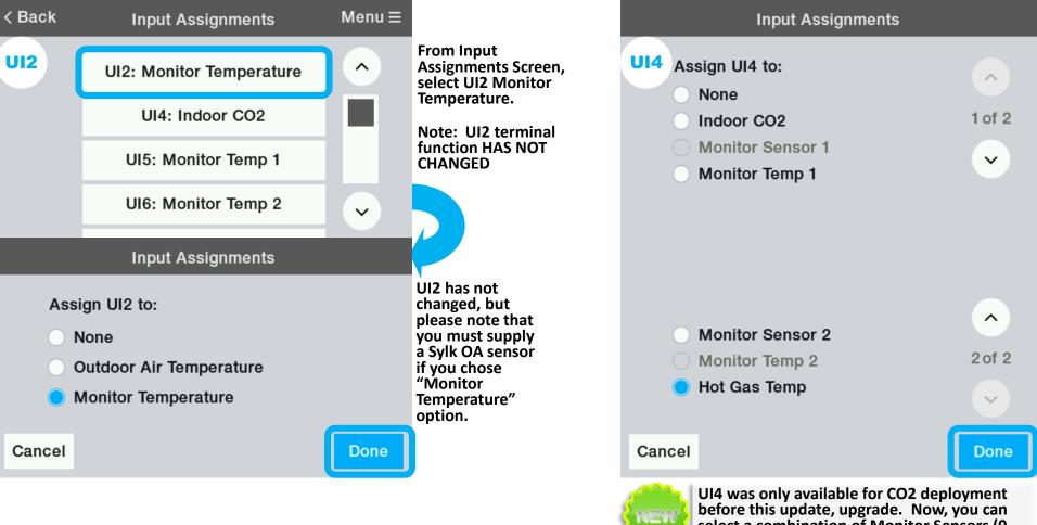
before this update, upgrade. Now, you can select a combination of Monitor Sensors (0-10 VDC) Monitor Temperatures (20K) and "Hot Gas Temp" that is designated for compressor discharge analytic.
