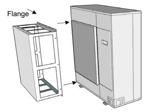
3. Carefully install the provided screws. Type-2 baffles have screw holes on the side of the baffle (in addition to the flange). If installing on a condensing unit with a square fan guard, also install screws through the baffle into the fan guard for added support.
