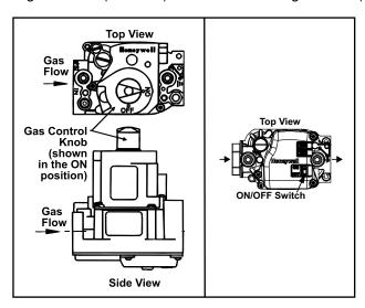
Figure 18. Gas Valve ON/OFF Control
