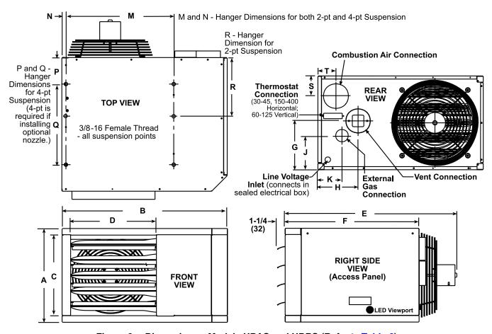
Figure 3. Dimensions—Models UDAS and UDBS (Refer to Table 6)
