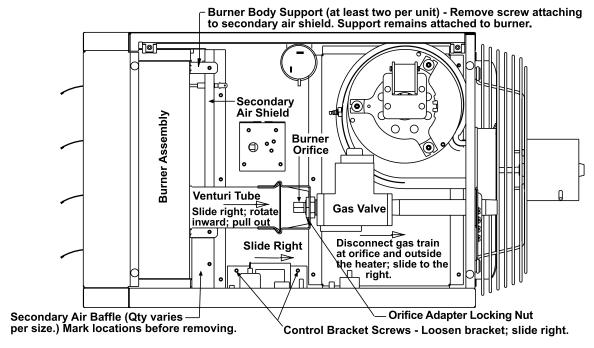
Figure 21. Burner Assembly (Typical View Shown)
