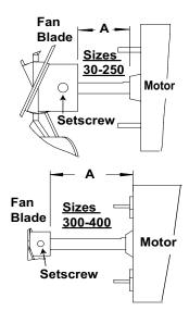
Figure 23. Fan Blade Positioning and Spacing
