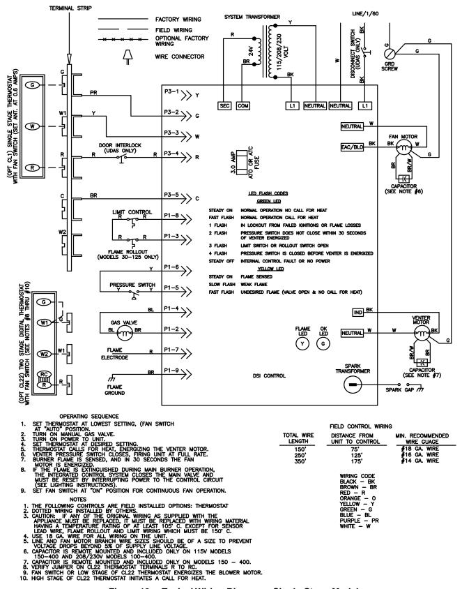
Figure 13. Typical Wiring Diagram—Single-Stage Models
