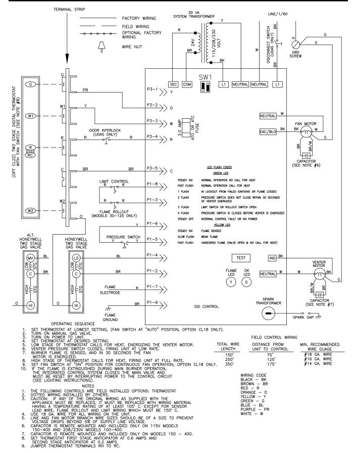
Figure 14. Typical Wiring Diagram—Two-Stage Models
