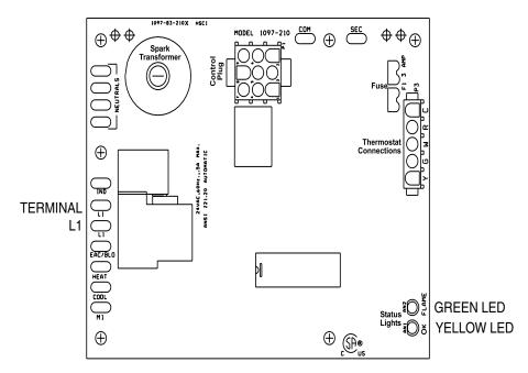
Figure 12. Circuit Board (DSI Integrated Control Module)
