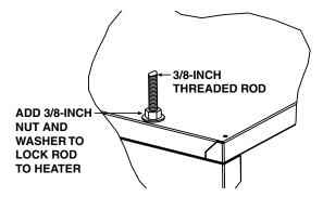
Figure 9. Heater Suspension Using Field-Supplied Threaded Rods
