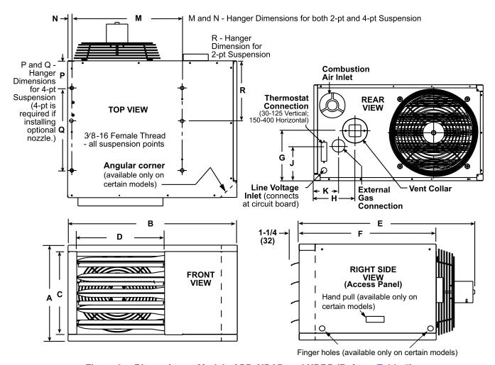
Figure 2. Dimensions—Models APD, UDAP, and UDBP (Refer to Table 5)
