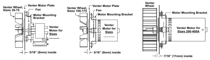
Figure 24. Venter Wheel Position on Shaft
