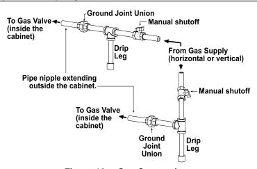
Figure 10. Gas Connections
