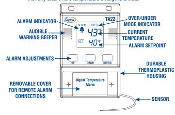
The TA22 Temperature Alarm is a single point or threshold type of temperature alarm. This type of temperature alarm monitors the temperature at the sensor probe tip and when this temperature passes above (or below) the set point, the unit will execute a preset operation.
