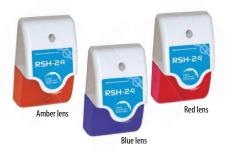
The Remote Strobe / Horn combines two alarm features, a visual and an audible into one compact, low profile device. It is powered by 24 VDC / VAC. The strobe and siren can be configured to activate together or each can activate separately from each other. It is recommended that this device be suitably mounted on a standard electrical box with conduit and protected from water ingress.
