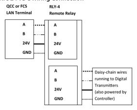
The RLY-4 can be wired directly to the QCC or FCS followed by digital transmitters connected in a daisy-chain configuration. Or it can be wired anywhere along the digital network in a daisy-chain configuration as required.
