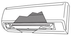
Cutaway view of typical Mini UV LED® installation in mini split
