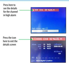
The details screen allows you to view the alarm level setpoints, priorities it is assigned to, the type of fault, when it was last calibrated, its Modbus® ID, and a description of the location of the transmitter for that particular channel.
