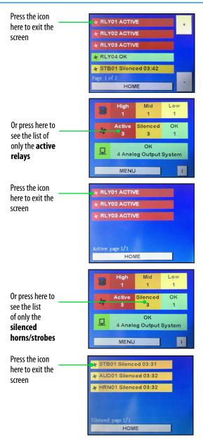
The status of a relay, horn, strobe or audible is indicated by colours and text added to the end of the line as follows:
