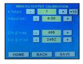
Use the + or - buttons or press the yellow fields and use the keypad to change the values, for each analog output. You can select:
