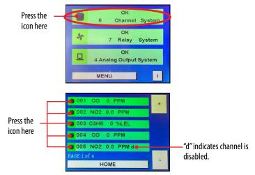
Use the + or - buttons to scroll to the channel you want to look at and press on icon on the bar for the particular channel of interest:
