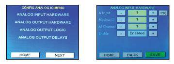
The maximum number of combined analog output devices the FCS-8 can accommodate is: 4 internal + 1 LNK-AO + 4 Modbus VFDs
