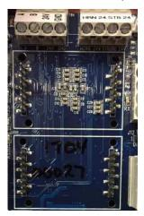
FCS main board without the optional Analog Input (-AI) or Analog Output (-AO) boards installed.
