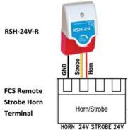
As shown, Strobe & Horn operate together.
