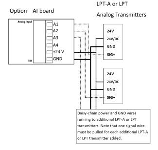
**NOTE:** DO NOT USE solid-core wire for connection to wiring terminal strip. Any damage caused by using solid-core wire will void warranty. Use stranded wire pigtails 18 awg within the enclousre to connect to the circuit board. The rigidity of solid-core wire can pull a soldered terminal strip completely off a circuit board and this will not be covered under warranty.
