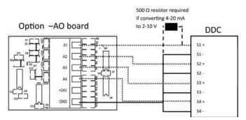
**NOTE:** DO NOT USE solid-core wire for connection to wiring terminal strip. Any damage caused by using solid-core wire will void warranty. Use stranded wire pigtails 18 awg within the enclosure to connect to the circuit board. The rigidity of solid-core wire can pull a soldered terminal strip completely off a circuit board and this will not be covered under warranty.
