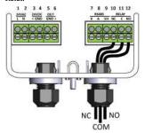
**NOTE:** The relay can be programed to be failsafe (normally energized). By default, the relay is set to be normally de-energized. This can be set using parameter P-06.
