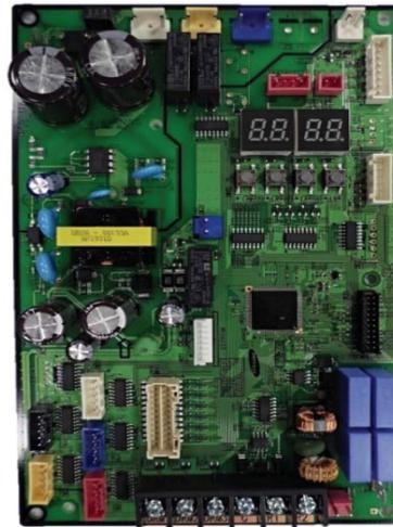
1. Turn on the outdoor unit, and then check whether the display 1/2 indications are displayed "E199" code.
