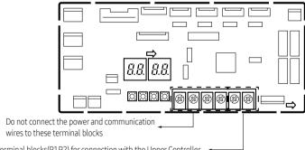
Terminal blocks(R1,R2) for connection with the Upper Controller (DMS, Touch, On/Off Controller, etc.)
