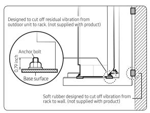
Install a proper grommet in order to reduce noise and residual vibration transferred by the outdoor unit towards the wall.
