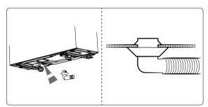
**4** Be sure to plug the rest of drain holes not connected with drain plugs using drain caps.
