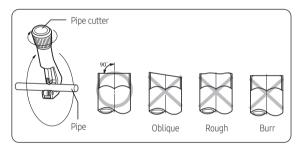
To prevent a gas leak, remove all burrs at the cut edge of the pipe using a reamer.
