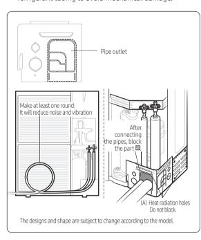
The refrigerant pipe can be pulled out from front, side, rear and bottom side, so install it depending on the installation site condition.
